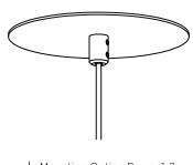
Mounting Option Power 1-2 Octagon Box (By Others) Installed in drywall, wood or concrete ceiling
